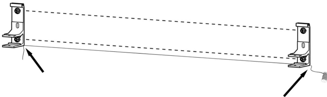
10) Slide the awning on wall brackets so that the construction is maximally pressed to the back (Note – before placing the awning verify the alignment of brackets – wall surface should be of the same thickness at installation spots).
