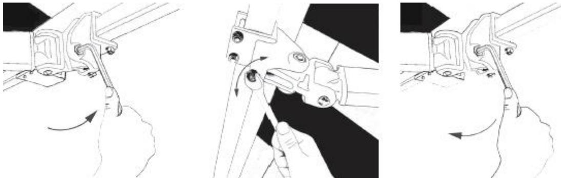
16) If necessary, modify the roller tube bracket position after changing the tilt angle.
